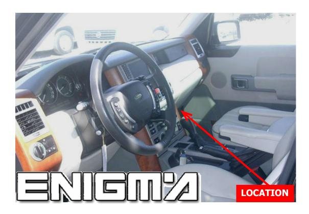
Use cable C12, remove module from car, open it completely, when we have board on our hands, connect or solder cable leads according to poitns shown into photo:
