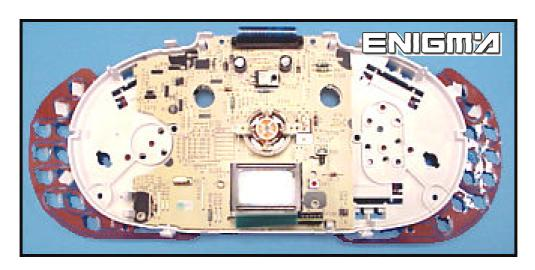
THEN REMOVE MAIN BOARD AND LOCATE EPROM 93C46 MEMORY, CLIP IT CHECKING PIN 1 AS SHOWN OF PHOTO BELOW:
