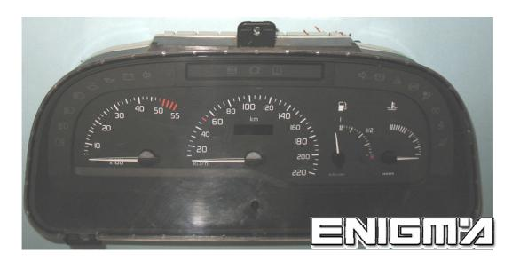
USE CABLE C8 - ST62XX, REMOVE BACK COVER FROM DASH, THEN REMOVE MAIN BOARD, JUST PULL IT OFF. NOW TAKE SCREEN BOARD AND THEN SOLDER CABLE LEADS ACCORDING TO ITS COLOUR LIKE WE CAN SEE ON NEXT PHOTO:
