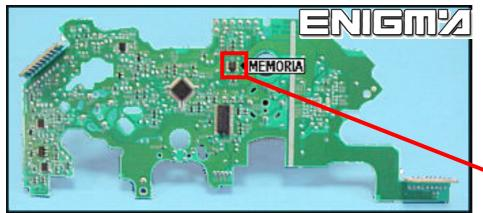
LOCATE EPROM 93C46, CLIP IT CHECKING PIN 1 AS SHOWN OF PHOTO:
