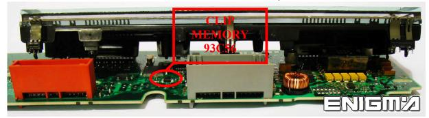
WE CAN CLIP DIRECT EPROM USING CABLE C4, OR USE CABLE C7, IN THIS CASE SOLDER CABLE LEADS LIKE PHOTOS SHOWN TO US:
