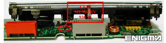
We can clip direct eprom using cable C4, or use cable C7, in this case solder cable leads like photos shown to us:
