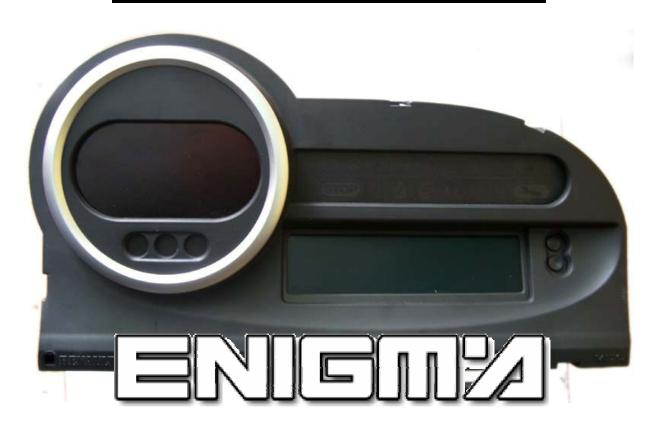
Use cable **C4**, open all dash, please make it carefully when touch screen, then locate eprom memory **93C56**, we don't need to desolder it, and clip it checking pin 1 as shown of photo below:
