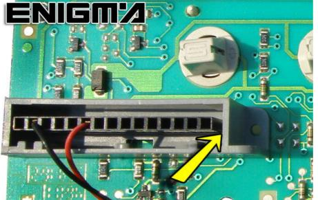
USE SPECIFIC CABLE C42. WHEN BOARD IS ON OUR HANDS, CONNECT PLUG TO DASH LIKE WE CAN SEE ON NEXT PHOTO, THIS IS THE POWER:
