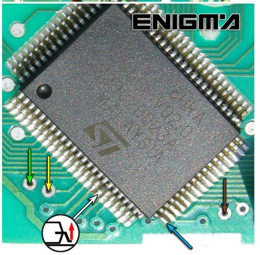
THEN CONNECT OR SOLDER CABLE LEADS ACCORDING TO COLOURS AS SHOWN ON THE PHOTO, PLEASE REMEMBER TO LIFT UP PIN FROM WHITE LEAD:
