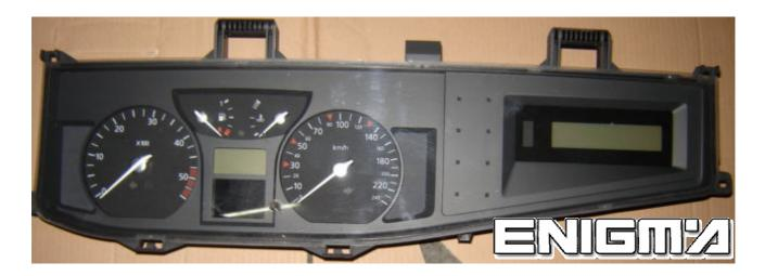
USE SPECIFIC CABLE C27, TAKE OFF BACK COVER FROM DASH, THEN CONNECT POWER SUPPLY PLUG INTO SOCKET AND SOLDER OR CONNECT CABLE LEADS ACCORDING TO COLOURS AS SHOWN OF BELOW PHOTO:
