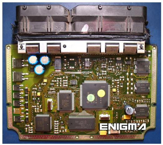
THEN LOCATE EPROM MEMORY 24CO4, AND CLIP IT CHECKING PIN 1 AS SHOWN OF BELOW PHOTO:
