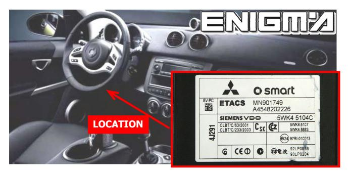
USE CABLE C12, LOCATE MODUL, BACK OF FUSES BOX, REMOVE IT, OPEN ALL CAREFULLY, THEN CONNECT OR SOLDER CABLE LEADS ACCORDING TO COLOUR AS SHOWN OF PHOTO BELOW:
