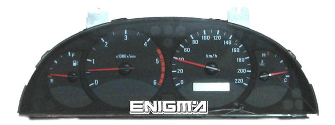
USE CABLE C4, OPEN BACK PLASTIC COVER FROM DASH, THEN LOCATE EPROM 93C46 MEMORY, AND CLIP IT CHECKING PIN 1 AS SHOWN OF BELOW PHOTO:
