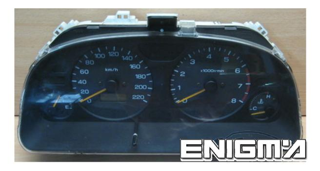
USE C4 CABLE, TAKE OFF ONLY SPEDOMETER, IT IS THE SCREEN ONE, THEN WE CAN SEE THE 93C46 EPROM, AND WITH THE PHOTO BELOW WE CAN CLIP MEMORY OR WE CAN CHOOSE TO MAKE BY BACK SOLDERING CABLE FOR IT C7:
