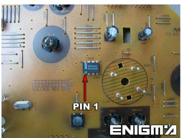
USE CABLE C5, OPEN ALL DASH, PLEASE MAKE IT CAREFULLY, THEN LOCATE EPROM MEMORY 93C56, USUALLY WE DON'T NEED TO DESOLDER IT, AND CLIP IT CHECKING PIN 1 AS SHOWN OF PHOTO:
