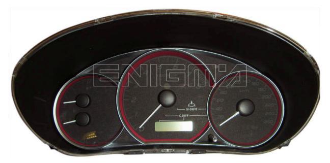
USE CABLE C4, REMOVE BACK PLASTIC COVER FROM DASH, PLEASE MAKE IT CAREFULLY, THEN LOCATE EEPROM MEMORY AND CLIP IT CHECKING PIN 1 AS SHOWN ON PHOTO BELOW:
