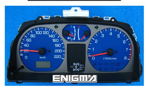
USE C7 CABLE, REMOVE ONLY SPEEDOMETER, IT IS THE SCREEN ONE, THEN WE CAN SEE THE 93C46 EPROM, AND WITH THE PHOTO BELOW WE CAN CLIP MEMORY OR WE CAN CHOOSE TO MAKE BY BACK SOLDERING CABLE FOR IT C7:
