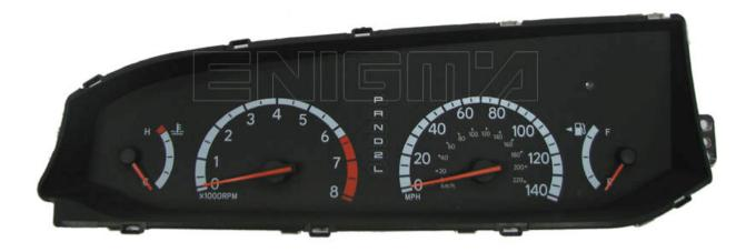
USE CABLE C5, OPEN CAREFULLY ALL DASH, THEN LOCATE EPROM 93C46 MEMORY, AND CLIP IT CHECKING PIN 1 AS SHOWN OF BELOW PHOTO:
