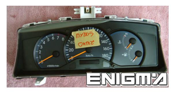
USE CABLE C5, REMOVE BACK PLASTIC COVER FROM DASH, THEN LOCATE EPROM 93C46, AND CLIP IT CHECKING PIN 1 AS SHOWN ON PHOTO BELOW:
