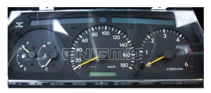
USE CABLE C4, REMOVE BACK PLASTIC COVER FROM DASH, AND THEN LOCATE EPROM MEMORY, AND CLIP IT CHECKING PIN 1 AS SHOWN ON PHOTO BELOW:
