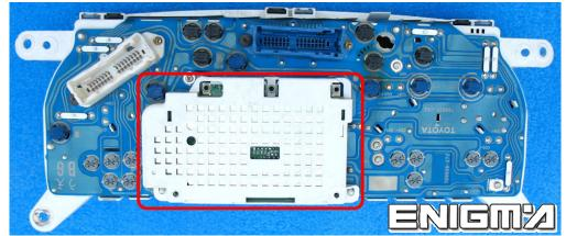
OPEN AND LOCATE EPROM 93C56, SOMETIMES MUST BE CLENED, AND CLIP IT CHECKING PIN 1 AS SHOWN IN THE PHOTO BELOW:
