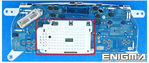
OPEN IT AND LOCATE POINTS ON THE BOARD, AND THEN SOLDER CABLE LEADS CONCORDANCE WITH ITS NUMBER-COLOUR:
