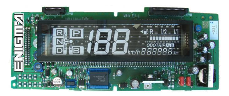
Use cable C7, remove dash from car, it can take you some time... Open dash, and then locate points in the main board like in photo below and solder cable leads as it shows to us:
