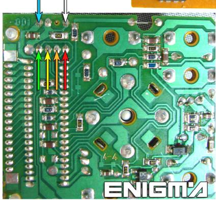
YOU CAN ALSO USE C7 CABLE, WE ONLY NEED TO LOCATE POINTS IN THE MAIN BOARD LIKE IN PHOTO AND SOLDER CABLE LEADS AS IT SHOWS TO US:
