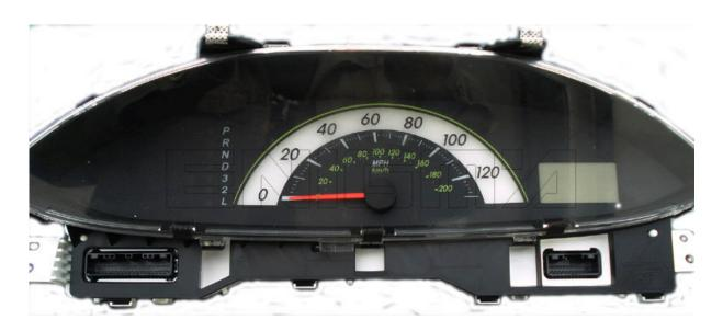
USE CABLE C4, OPEN DASH, PLEASE MAKE IT CAREFULLY, THEN LOCATE EEPROM C46 MEMORY AND CLIP IT CHECKING PIN 1 AS SHOWN OF PHOTO BELOW:
