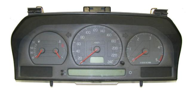
USE CABLE C4, REMOVE BACK PLASTIC COVER OF DASH, CAREFULLY, THEN PULL OUT MAIN BOARD, LOCATE EPROM 93C56, SOMETIMES NEED TO BE CLEANED, AND CLIP IT CHECKING PIN 1 AS SHOWN OF BELOW PHOTO:
