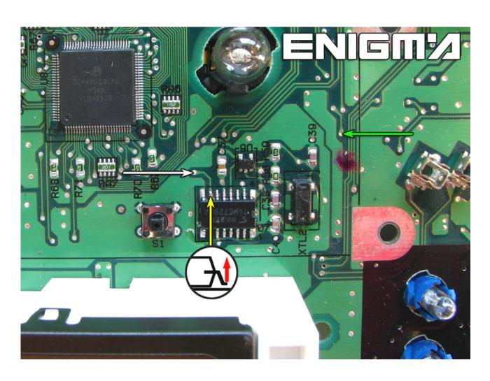
THEN CONNECT GROUND AND POSITIVE CABLE (BLACK AND RED) LIKE WE CAN SEE ON NEXT PHOTO AND MAKE BRIDGE BETWEEN ELEMENT L6 AND TRANSISTOR TR1 (SHOWN BY ORANGE LINE ON SECOND PHOTO). AFTER SOLDERING CONNECT CABLE C12 TO ENIGMA AND IN MENU SELECT VOLVO V70 HC08.
