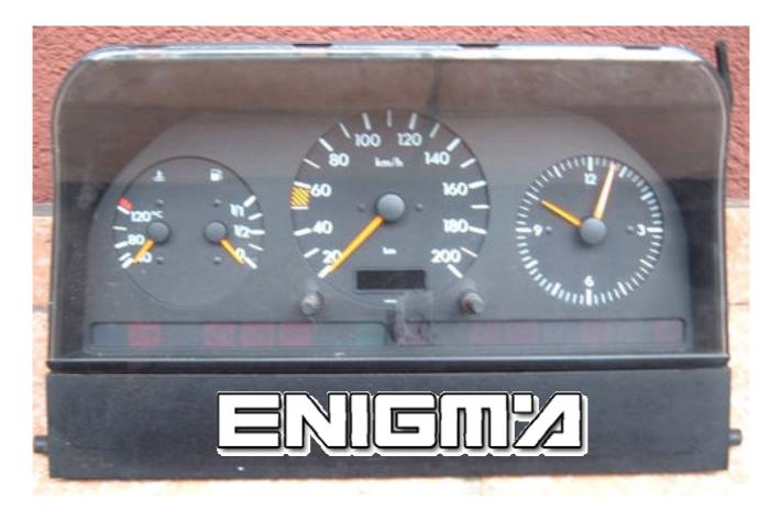
USE SPECIFIC CABLE C32, REMOVE DASH FROM CAR, CONNECT PLUG TO DASH LIKE WE CAN SEE ON NEXT PHOTO AND RUN PROGRAM:
