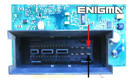
Now locate points on the other side of board like in photo below and solder cable leads as it shows to us:
