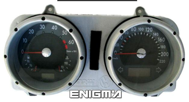
USE CABLE C4, OPEN DASH, PLEASE MAKE IT CAREFULLY, THEN LOCATE EEPROM 24CO4 MEMORY AND CLIP IT CHECKING PIN 1 AS SHOWN OF PHOTO BELOW:
