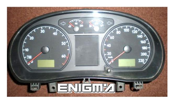
USE CABLE C12 O HCS12, REMOVE BACK COVER FROM DASH, THEN CONNECT OR SOLDER CABLE LEADS ACCORDING TO COLOURS AS SHOWN OF BELOW PHOTO:
