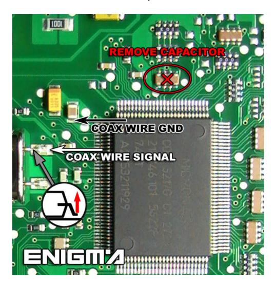
Now locate points on the other side of board like in photo below and solder cable leads as it shows to us:
