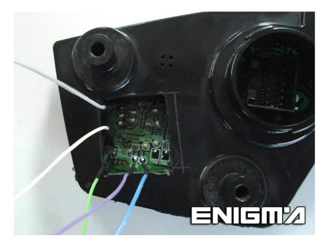
USE C7 CABLE, LOCATE POINTS IN THE MAIN BOARD LIKE IN PHOTO BELOW AND SOLDER CABLE LEADS AS IT SHOWS TO US:
