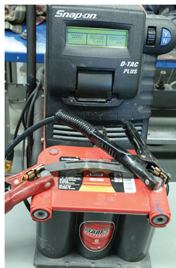
FIGURE 6-2 A battery with 12.4V or less should be tested and, if OK, charged to 100% using a “Smart” charging system.
