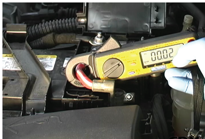
FIGURE 6-16 Low-amps probe hooked up to battery cable.
