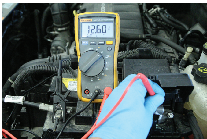
FIGURE 6-1 Source voltage is measured at the battery and should be very close to 12.6 volts.
