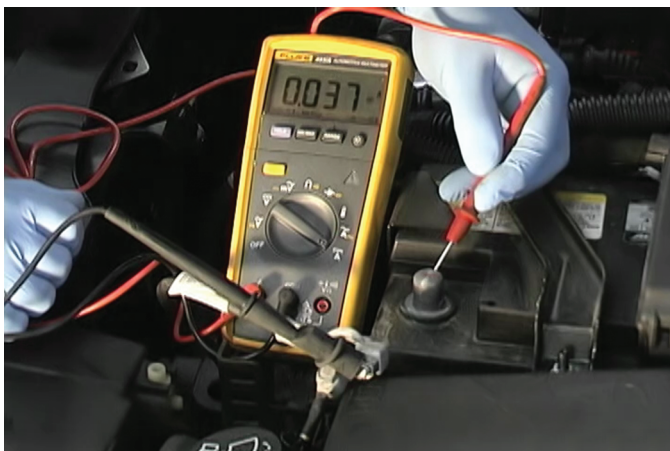
FIGURE 6-14 The parasitic draw test determines the amount of current used by systems when the vehicle is off.
