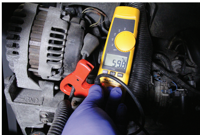
FIGURE 6-8 An inductive clamp can be used to measure amperage values that exceed the limit of the DMM or if you want to view the signal on a DSO.
