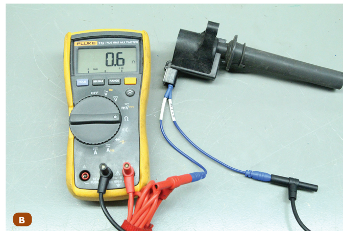
FIGURE 6-6 A resistance test can determine if a component is within service information specifications.
