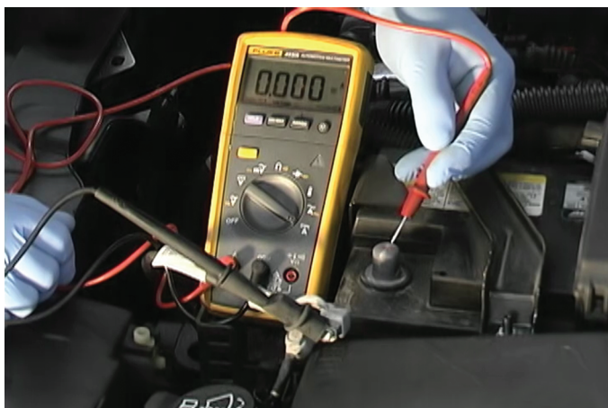
FIGURE 6-15 DMM hooked up to measure parasitic draw.
