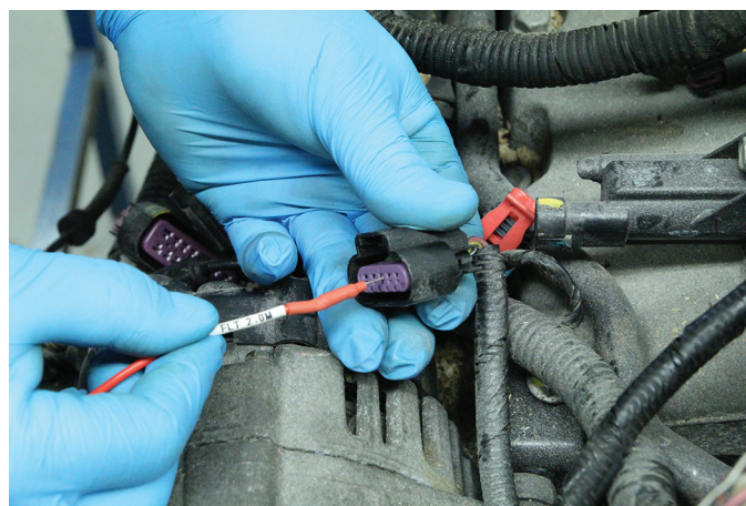
FIGURE 6-18 Terminal pin test tools can be used to verify the correct pin fit tension is present.
