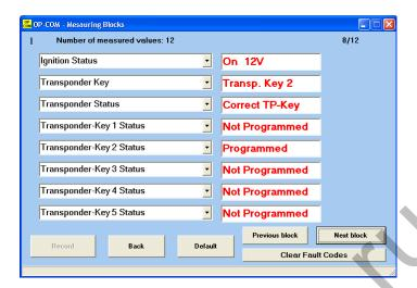
The immobiliser and the Engine ECU is connected together via a W-Line. (W comes from a german word, WegfahrSperre=Immobiliser)
