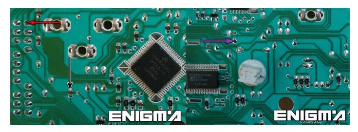
AND FINALLY SOLDER CABLE LEADS ACCORDING TO COLOURS AS SHOWN OF BELOW PHOTO (REMEMBER TO LIFT UP ONE PIN 21 FROM MICROCONTROLLER):
