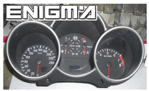
USE CABLE C13 ALWAYS CONNECTED TO A1 ADAPTER. OPEN COMPLETELY DASH, BE CAREFULLY WITH SCREEN, THEN CONNECT OR SOLDER CABLE LEADS ACCORDING TO NUMBER AS SHOWN IN NEXT PHOTO:
