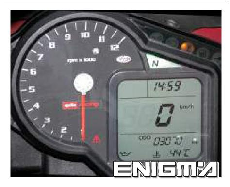
Use cable C4, open all dash carefully, remove screen and don't touch nail, then move plastic chassis and look for eprom 24CO2, when we have it in front of us clip it checking Pin 1 as shown of photo below:
