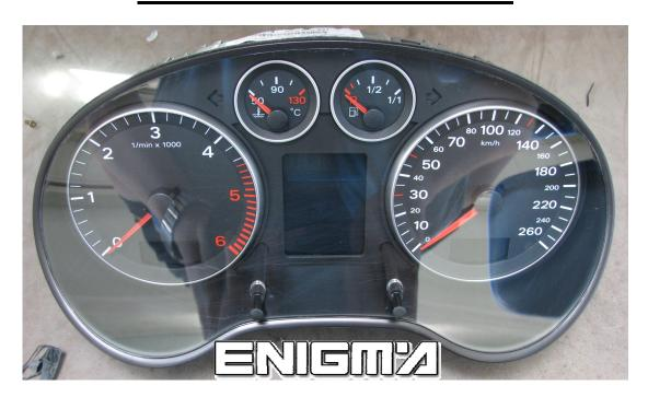
USE CABLE C44 + A5 ADAPTER, REMOVE DASH FROM CAR AND OPEN IT COMPLETELY. SEPARATE BOTH BOARDS FROM DASH, AND CONNECT POWER ON PLUG:
