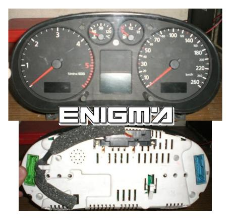
THIS KIND OF DASHBOARDS USUALLY WORKS BY DIAGNOSIS(OBD2), BUT SOME VERSIONS CAN NOT WORK AND WE MUST REMOVE DASH FROM CAR, THEN USING C12 CABLE, OPEN BACK PLASTIC COVER OF DASH, THEN LOCATE POINTS, AND SOLDER CABLE LEADS ACCORDING TO COLOURS AS SHOWN OF BELOW PHOTO:
