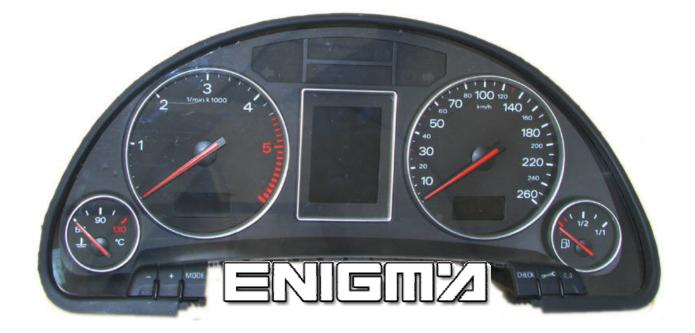
THIS KIND OF DASHBOARDS USUALLY WORKS BY DIAGNOSIS, BUT SOME VERSIONS CAN NOT WORK AND WE MUST REMOVE DASH FROM CAR, THEN USING C4, OPEN ALL DASH, PLEASE MAKE IT CAREFULLY, WE MUST REMOVE 2 NAILS AND SCREEN, JOB IS NOT A BIG PROBLEM. THEN LOCATE EEPROM 24C08 MEMORY AND CLIP IT CHECKING PIN 1 AS SHOWN OF PHOTO BELOW:
