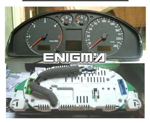
THIS KIND OF DASHBOARDS USUALLY WORKS BY DIAGNOSIS, BUT SOME VERSIONS CAN NOT WORK AND WE MUST REMOVE DASH FROM CAR, THEN USING C12 CABLE, OPEN BACK PLASTIC COVER OF DASH, THEN LOCATE POINTS, AND SOLDER CABLE LEADS ACCORDING TO COLOURS AS SHOWN OF BELOW PHOTO:
