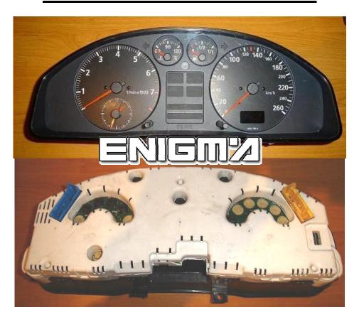
USE CABLE C4, OPEN ALL DASH, TO REMOVE MAIN BOARD YOU SHOULD TAKE OFF ENGINES SCREWS, THEN LOCATE EPROM, SOMETIMES MUST BE CLEANED, AND CLIP IT CHECKING PIN 1 AS SHOWN OF BELOW PHOTO:
