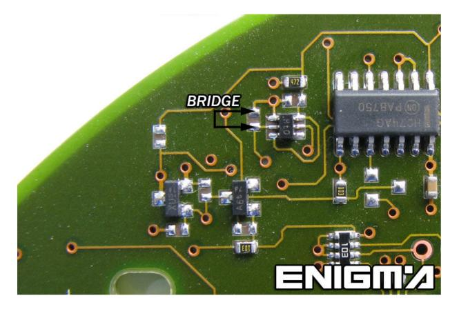
USE CABLE C46, REMOVE DASH FROM CAR AND OPEN BACK PLASTIC COVER. CONNECT POWER PLUG. NOW LOCATE POINTS ON THE BOARD LIKE IN PHOTO BELOW AND SOLDER CABLE LEADS AS IT SHOWS TO US:
