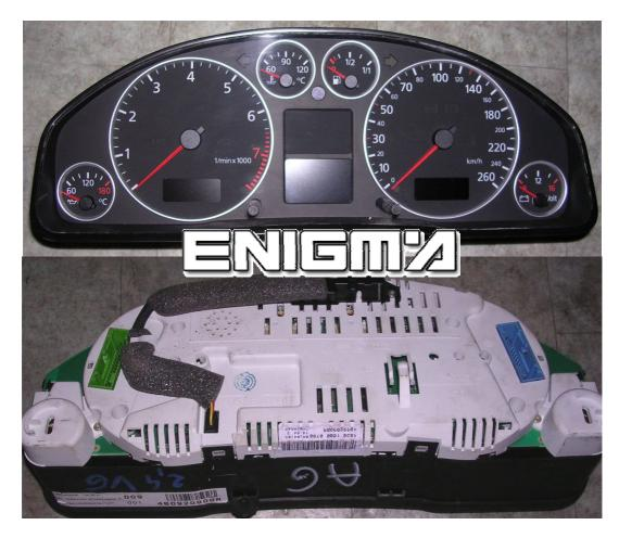
THIS KIND OF DASHBOARDS USUALLY WORKS BY DIAGNOSIS, BUT SOME VERSIONS CAN NOT WORK AND WE MUST REMOVE DASH FROM CAR, THEN USING C12 CABLE, OPEN BACK PLASTIC COVER OF DASH, THEN LOCATE POINTS, AND SOLDER CABLE LEADS ACCORDING TO COLOURS AS SHOWN OF BELOW PHOTO:
