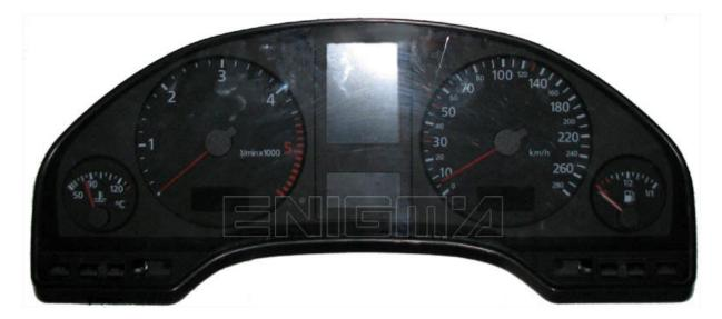
USE CABLE C4, OPEN BACK SIDE FROM DASH, WE MUST DISCONNECT TWO LITTLE PLUGS TO MAKE IT. THEN LOCATE EPROM 24C16 OR 24C17, CLIP IT CHECKING PIN 1, READ THE CORRECT VALUE, BECAUSE THERE ARE 2 DIFFERENT SOFTWARE VERSIONS, WITH THE CORRECT ONE WE WILL PROGRAM IT:
