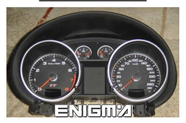
USE CABLE C44 + A5 ADAPTER, REMOVE DASH FROM CAR AND OPEN IT COMPLETELY. SEPARATE BOTH BOARDS FROM DASH, AND CONNECT POWER ON PLUG:
