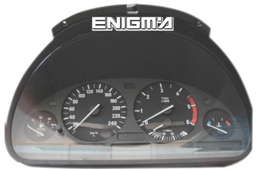
USE C7 CABLE, WE ONLY NEED REMOVE BACK COVER FROM DASH, LOCATE POINTS IN THE MAIN BOARD LIKE IN PHOTO BELOW AND SOLDER CABLE LEADS AS IT SHOWS TO US. NEVER TOUCH NAILS, IT IS VERY DANGEROUS. MEMORY INSIDE THESE KINDS OF CARS IS A M35080.
