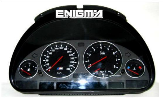
USE C7 CABLE, WE ONLY NEED REMOVE BACK COVER FROM DASH, LOCATE POINTS IN THE MAIN BOARD LIKE IN PHOTO BELOW AND SOLDER CABLE LEADS AS IT SHOWS TO US. NEVER TOUCH NAILS, IT IS VERY DANGEROUS. MEMORY INSIDE THESE KINDS OF CARS IS A M35080.
