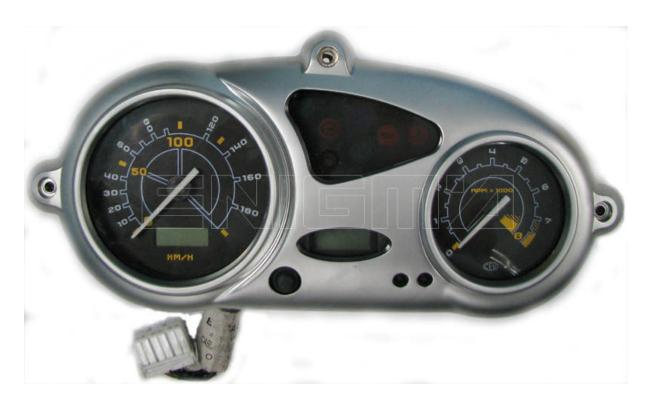
USE CABLE C4, OPEN ALL DASH, PLEASE MAKE IT CAREFULLY, THEN LOCATE EPROM MEMORY 93C56, USUALLY WE DON'T NEED TO DESOLDER IT, AND CLIP IT CHECKING PIN 1 AS SHOWN OF PHOTO BELOW:
