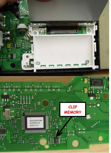
OPEN DASH COMPLETELY, CAREFULLY REMOVE SCREEN. CHECK THE PHOTO:
